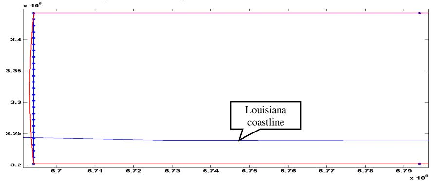
This slide exhibits the western boundary of the two perimetersin extreme aspect ratio. Asterisks are placed on the blueperimeter every 10km. The graphic is 240km high and 10kmwide. Notice the curvature of the red, reprojected Z14boundary. This curvature preserves orthogonality at the corners.12/15/2011Orthogonality Preserved v524
