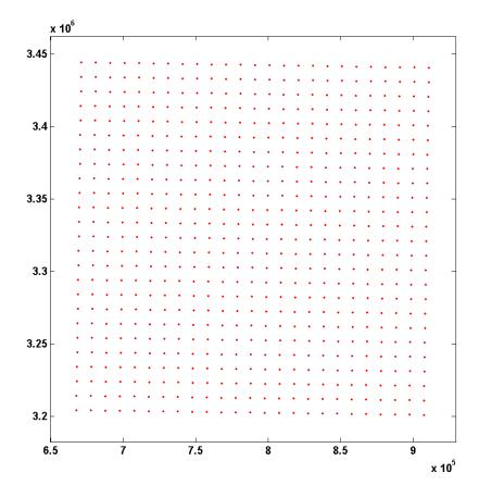
In segmented quadrilateral gridding the whole project polygon is subdivided (576 times in this case) and all vertices are reprojected cartographically. The bin centers are populated trigonometrically within each smaller quadrilateral.
