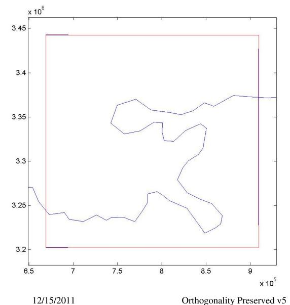
In this slide the reprojected Z14 red perimeter is rotated into best alignment with the original Z15 blue perimeter.
