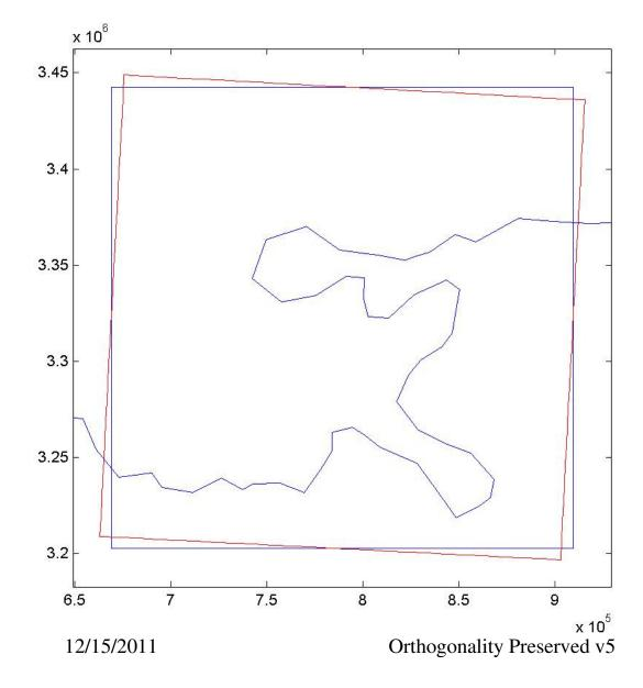
The blue (square) perimeter is the original Zone 15 AOI. The red perimeter is the AOI reprojected into Zone 14 then translated so that the centers of the two perimeters coincide. The difference in orientation is due to convergence of the meridians.
