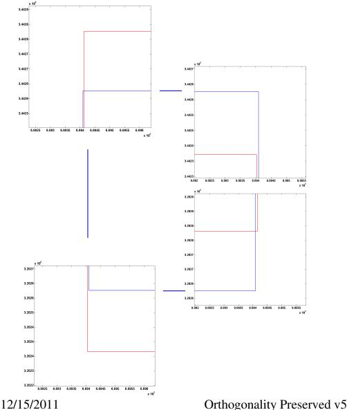
This slide exhibits close-up views of the four corners of the superimposed perimeters. The "trapezoidal" shape of the re-projected red Z14 perimeter is clearly seen. This is due to the varying point scale factor over the zone. All corners (blue and red) are orthogonal.
