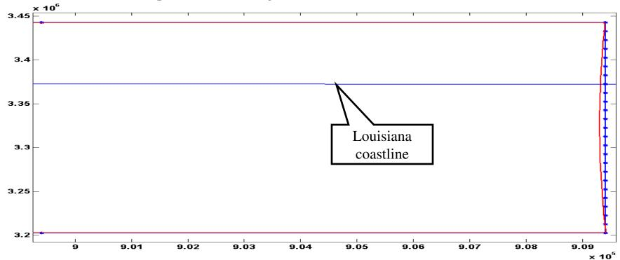
This slide exhibits the eastern boundary of the two perimetersin extreme aspect ratio. Asterisks are placed on the blueperimeter every 10km. The graphic is 240km high and 10kmwide. Notice the curvature of the red, re-projected Z14boundary. This curvature preserves orthogonality at the corners.12/15/2011Orthogonality Preserved v525
